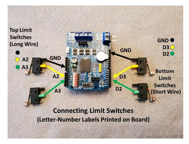
(2) The photo shows the connection on the Rover Driver Board on A2, A3, & GND to the Top Stepper Limit Switch Interface wires are marked as YELLOW, GEEN, & BLACK sleeves.
